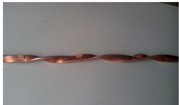
Fig.3 Copper square jagged Twisted tape (y=5.2) (Enlarged view)
